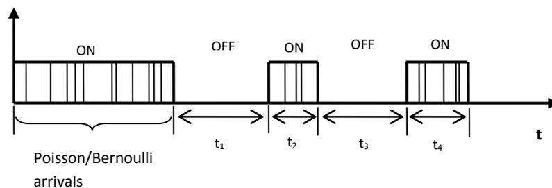
Fig 1: ON/OFF Traffic Model.
