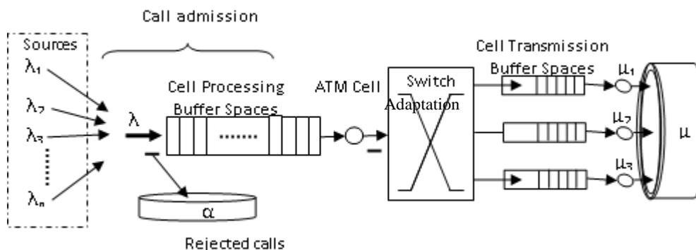
Figure 3: ATM network node model
